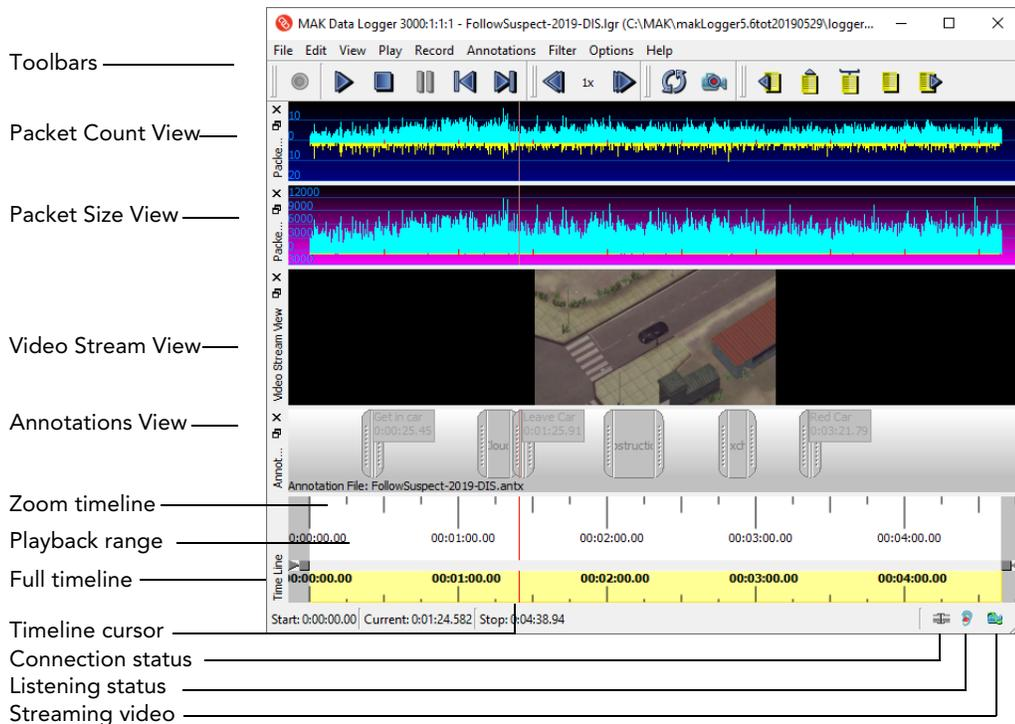
Figure 1-2. Logger window with a Logger file loaded
